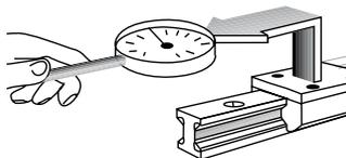
Tolerances in the guide system and internal friction may cause an increase of the slide resistance when the adjusted cassette is moved along the stroke path.
