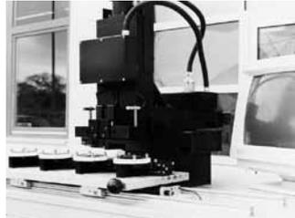
Aluminium roller guides in an automatic vibrator for flattening printed sheets of paper. To guarantee even pressure on the sheets of paper, the roller bridge is supported by precision roller guides. (Baumann company photo)
