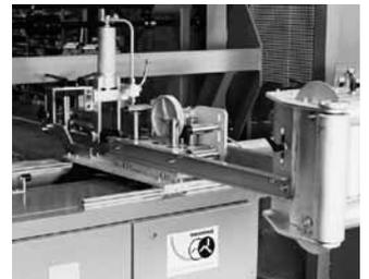
Single rail and roller shoe versions of the aluminium roller guide in a handling arrangement for stacks of paper. Various fittings and limit stops for stacking are moved on two axes horizontally and vertically. The robustness and reliability of the roller guides allows for continuous operation under high load conditions. (Solms company photo)
