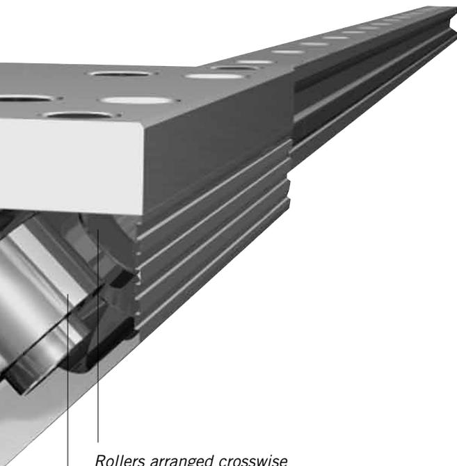
Rollers arranged crosswise to handle loading from any direction
