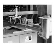
Single rail and roller shoe versions of the aluminium roller guide in a handling arrangement for stacks of paper. Various fittings and limit stops for stacking are moved on two axes horizontally and vertically.
