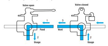
Removable lever: where the lever is obstructed in its movement, it can be refitted the opposite way.
