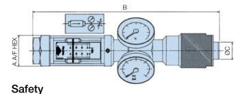
An axial flow restrictor valve is fitted which can be adjusted under full load from open to fully closed<sup>1</sup>, and to complete the specification, a safety blow-out disc, set to fail at 455 bar is fitted to the manifold in a position facing away from the operator when reading the gauges normally. Two spare blowout discs are supplied which are easily replaced by removing the hexagonal plug on the gauge manifold.
