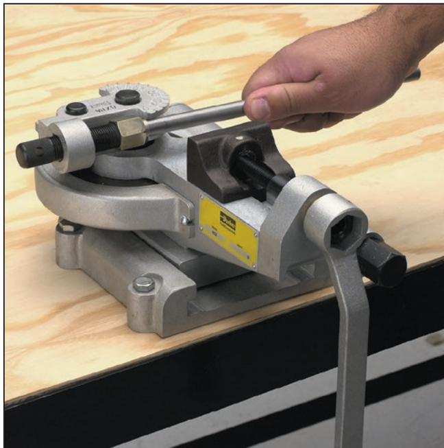
**Close Bend Radius Blocks** — The close bend radius blocks have a threaded pin which threads directly into both Triple-Lok and Ferulok tube fitting nuts. With the use of Parker's Seal-Lok close bend adapter, one can also use Seal-Lok fittings with a close bend radius block. They permit an operator to make his first bend very close to the end of the tube.
