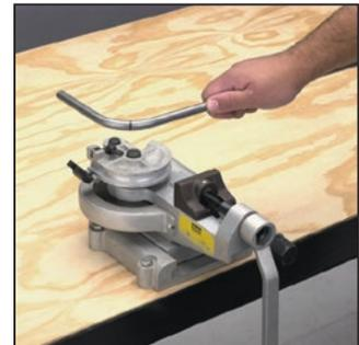
**Bends from 90° to 180°** — The 400 Series Tube Benders bend tubing up to 180° with ease. The procedure for bends over 90° is the same as for bends to 90°. See Step 4.
