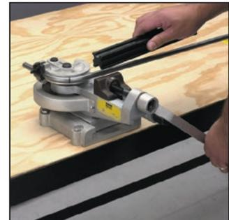
**Step 9: Completed Bent Tube**
