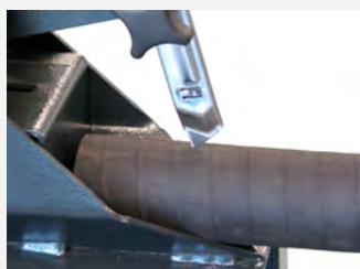
The SSG slitting tool shortens skiving chips
