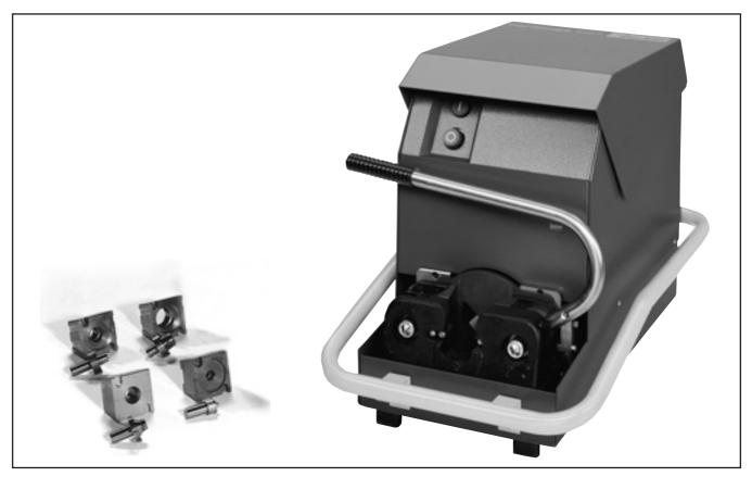
The Parflange® 1025 machine is designed to cold-form high pressure tube connections for O-Lok® and Triple-Lok® connection. It uses the Parflange® orbital flaring process. The Parflange® 1025 machine smoothly compresses the tube material and achieves a high strength joint with a polished surface of the tube end. O-Lok® and SAE flange sleeves are firmly fixed onto the tube end, resulting in a very rigid high-pressure tube connection.
