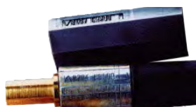
PTS SYSTEM Marking and crimping in one step according to DIN 20066, EN 853, EN 854, EN 856, EN 857 PTS 52: Zeichen/character 4 x 2,0 mm / marking depth ca. 0,3 - 0,5 mm PTS 32: character 3 x 1,5 mm / marking depth ca. 0,3 mm
