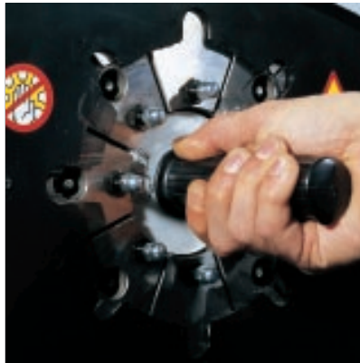
The head is closed and the dies are swaged together
