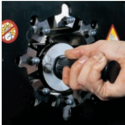
Die set is positioned inside the swaging head
